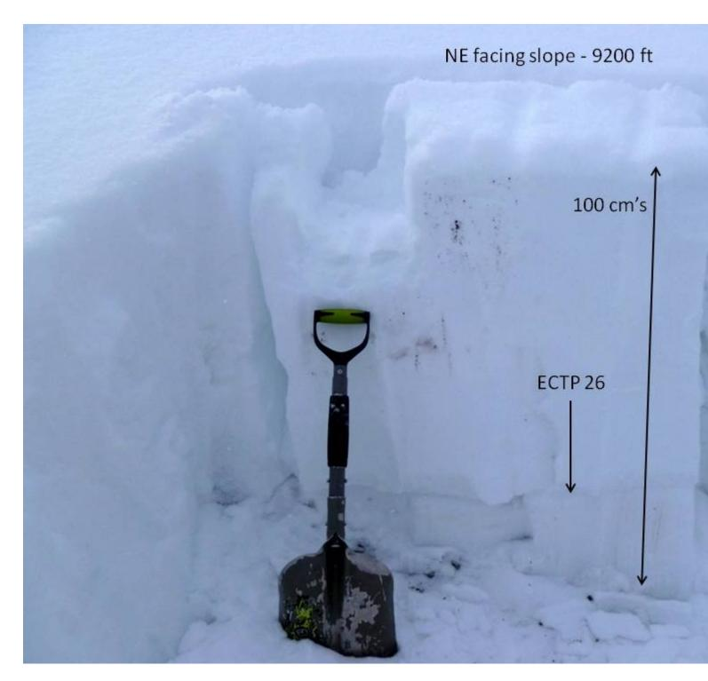
In the mountains north of West Yellowstone, facets near the ground produced unstable results during stability tests. This layer was found on a NE facing slope around 9200 ft, but was not found on a SE facing slope nearby. Before committing to steep avalanche terrain, digging to the ground to assess the strength and distribution of this layer is a good idea. Photo GNFAC
