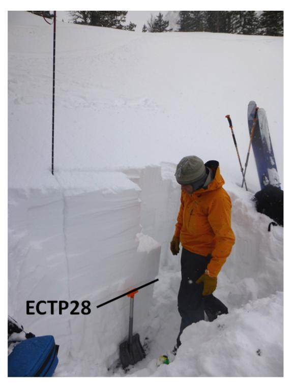
Mark Staples found 7 inches of dense (15%) new snow on a snowpack almost 5 feet deep. Two feet off the ground facets broke in the Extended Column Test. It's taking more force to get this layer to break, which is a sign of stengthening. Photo: GNFAC
