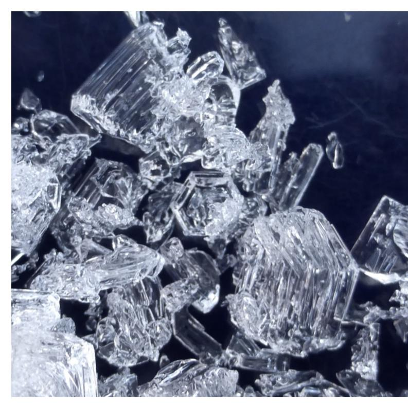
This weak layer was the weakest snow we have seen all season. Most places have square faceted crystals. This slope had large, cupped, striated, depth hoar crystals up to a centimeter in size. Photo: GNFAC
