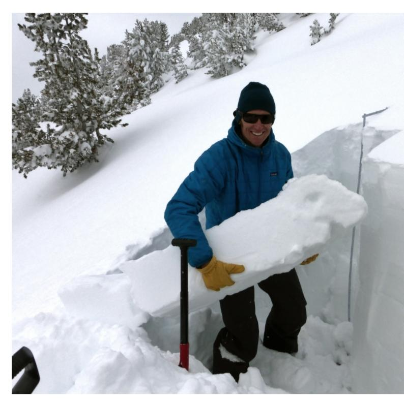
On a south facing slope on Scotch Bonnet Mtn north of Cooke City, there was no layer breaking in stability tests. Photo: GNFAC
