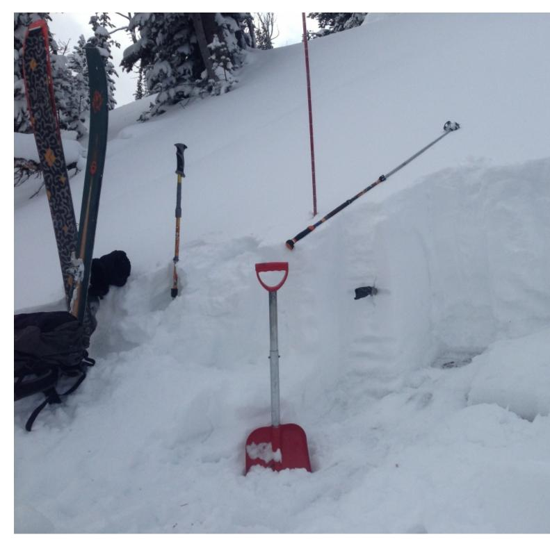
At 9,000 feet in Middle Basin/Beehive there's 2 feet of snow. Facets near the ground are breaking in some stability tests. This week's cold weather will likely allow the facets to grow bigger. Photo: A. Whitmore
